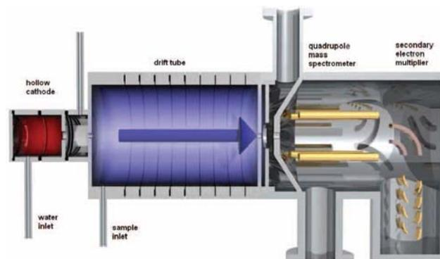
Figure 1. Schematic drawing of a PTR-MS apparatus. Hydronium ( $\text{H}_3\text{O}^+$ ), produced in a hollow cathode discharge region of the instrument, protonate the target VOC in the drift tube. The product ion is subsequently guided through a quadrupole mass filter and counted by a secondary electron multiplier detector.
